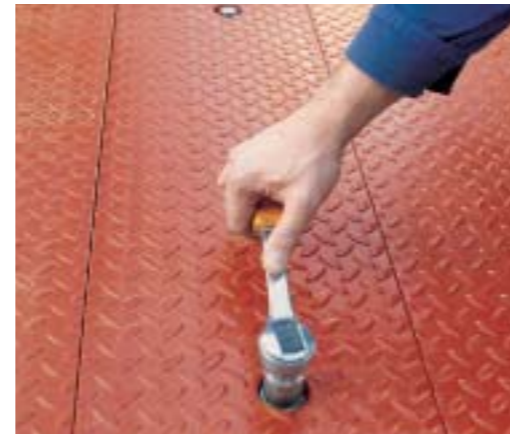
Inspection hatches ensure easy access to the load cells, even in the pit-mounted version.
