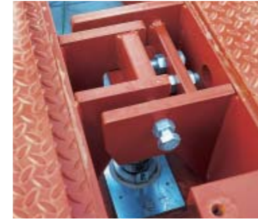
The "isostatic" panel connection system ensures that the weighbridge function correctly even when ground level varies between the different support points.
