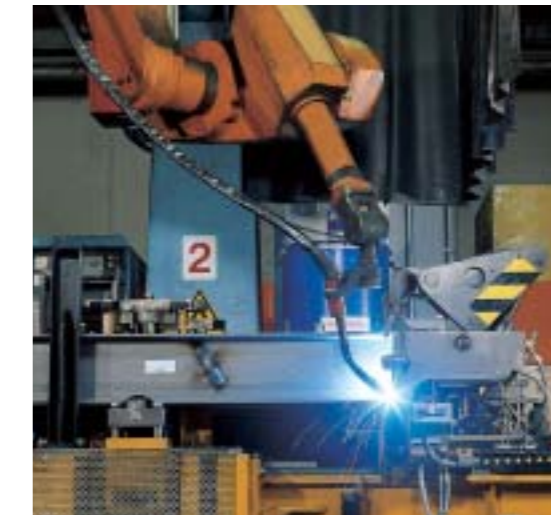
Robotic welding systems ensure perfect welds of a consistently high quality
