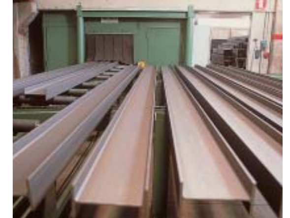
Automatic sandblasting line: all steel sections undergo sandblasting and linearity checks
