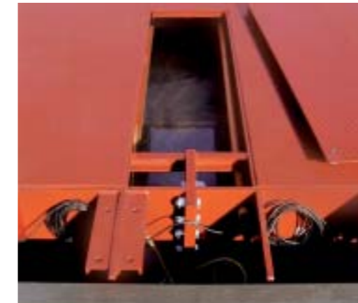
Centrally-positioned hatches facilitate cleaning operations.
