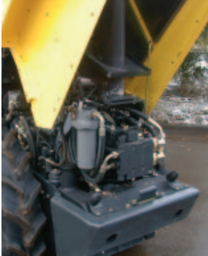
Locking, two (2) position engine hood opens to provide access to the reverse positioned engine, all critical components and maintenance items.
