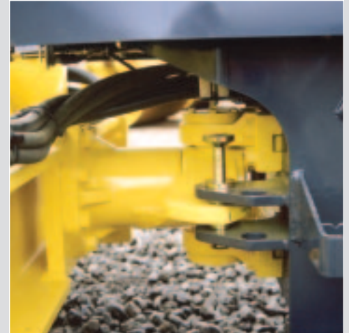
Bolt-on centerjoint is maintenance-free, providing optimum steering and oscillation angles.
