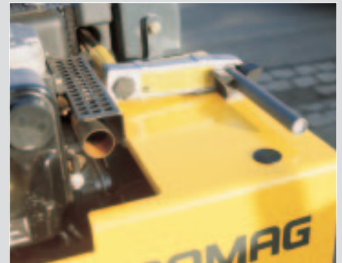
The safety starting handle is easily accessible
