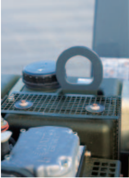
Balanced central lifting eye ensures safe and easy transportation
