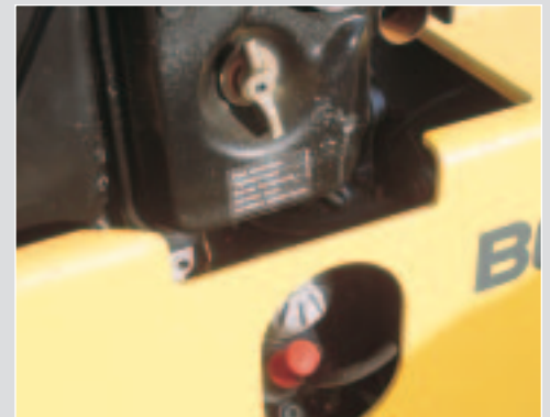
The oil level gauge and air filter are easily accessible for maintenance
