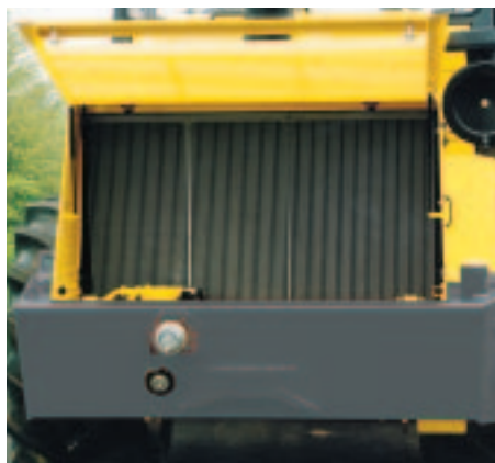
Simple access to the radiators makes cleaning easier
